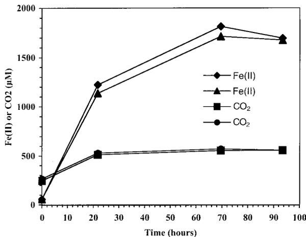
FIGURE 2. Respiration of structural Fe(II) and production of  $\Sigma\text{CO}_2$  in the same duplicate MR-1 cultures in a minimal medium with clay added as the sole electron acceptor and lactate added as the sole electron donor. Smectite was added to  $7.5 \text{ g L}^{-1}$ . Each value is the average calculated from duplicate cultures and measurements ranged less than 5% from the average of duplicates. Control cultures showed similar results to those found in Figure 1.
