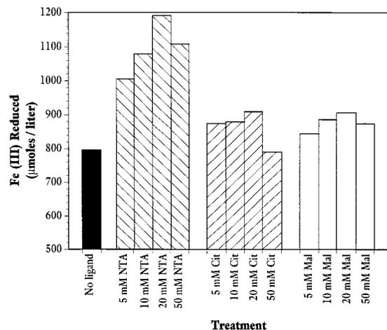
**FIGURE 3. Reduction of clay-bound Fe(III) after 1 week in duplicate MR-1 cultures containing a range of organic ligand concentrations. Smectite was added to 2.0 g L<sup>-1</sup>. Each value is the average calculated from at least duplicate cultures and measurements ranged less than 5% from the average of duplicates.**
